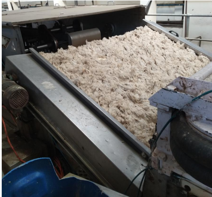
Photo: Wool fibre scouring (after scouring in first Bowl the fibres are squeezed and forwardd to second Bowl)
